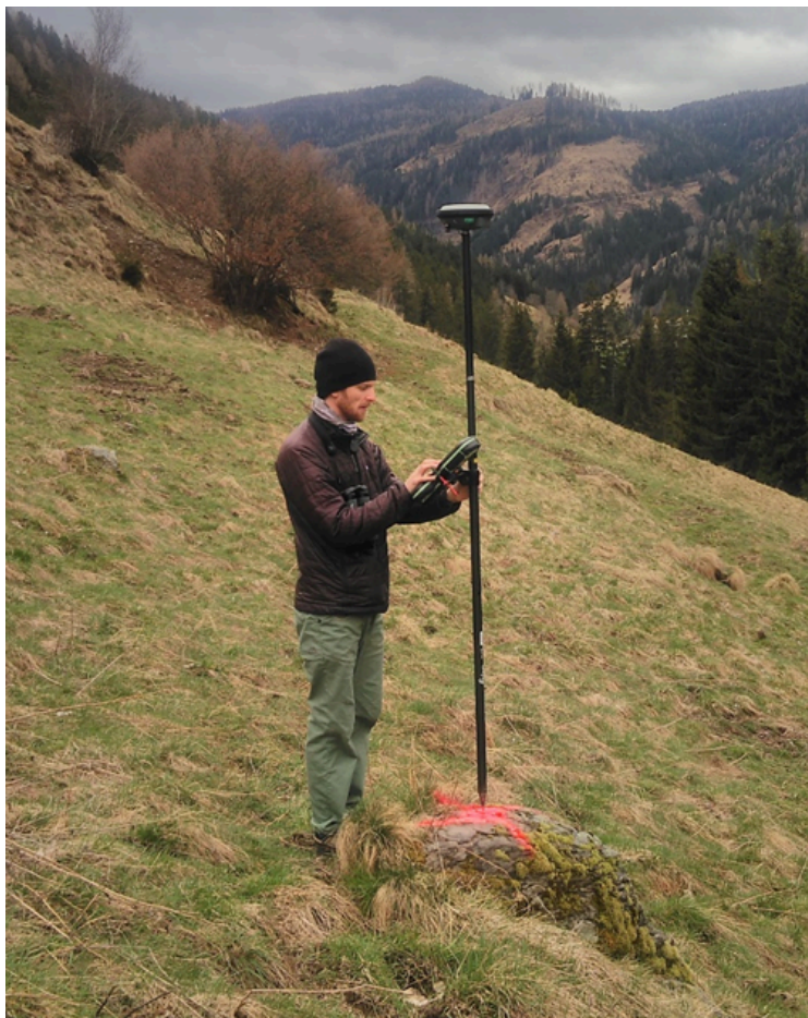
Figure g. Collecting GCP measurements at the study site Winkl, district of Feldkirchen, Carinthia, Austria using the Leica GS16 GNSS Rover
