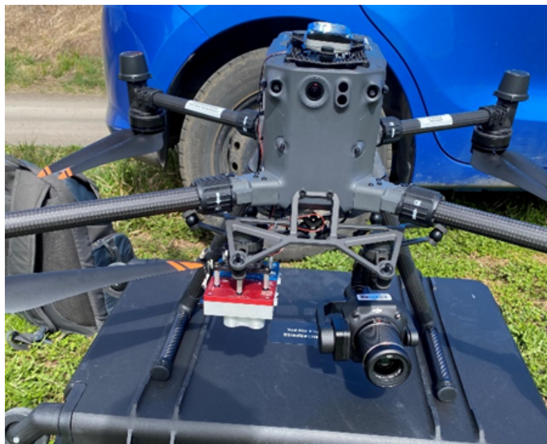
Figure h. The DJI M350 RTK is equipped with a Micasense dual (viewed from the front) on the left and a DJI P1 RGB camera mounted on the right. Both sensors are triggered at the same time.
